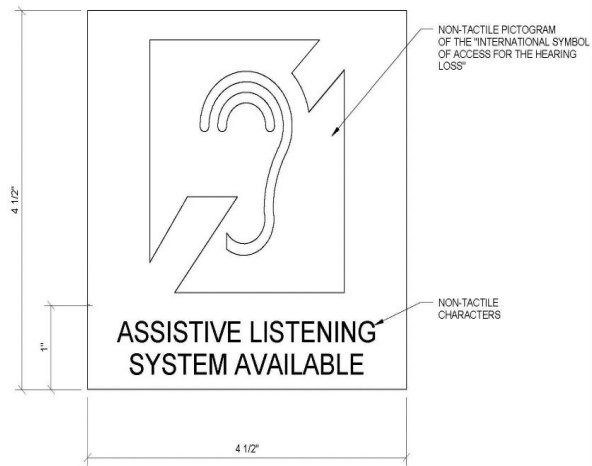
TYPE 2-D SIGNAGE NON-TACTILE CHARACTERS AND NON-TACTILE PICTOGRAM. PICTOGRAM TO BE THE INTERNATIONAL SYMBOL OF ACCESS FOR THE HEARING LOSS.
